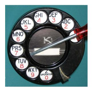
To lock the ring in place insert a small screwdriver or knife blade between the ring and the plastic window, slide the lock tab clockwise to between 6-5. To remove the ring insert the tool between 6-5 and slide the tab counterclockwise to 6-7 and then the ring can be lifted out from the left side.
