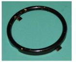
The locking lever engages the internal tab shown here (I-r) from the back of the ring and the front. The external tab fits a slot in the finger wheel between the O-1 position to the right of the finger stop.
