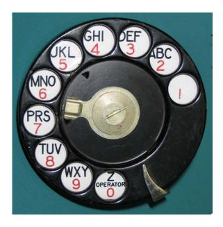
A locking lever is attached to the dial hub which moves between the 6-7 position (unlocked) and the 5-6 position (locked).
