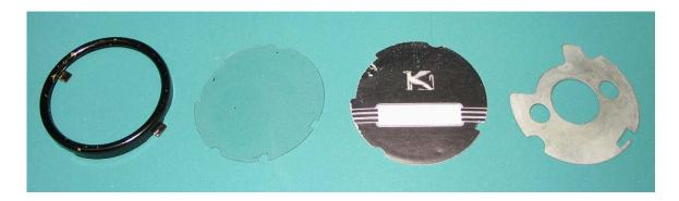
The dial card is assembled as shown left to right; the notch in the four o'clock position of the window and card fits a tab (shown in the left picture at the top in the two o'clock position) and insures that the card is positioned correctly when installed on the dial.
