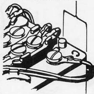
Figure 3. Recommended method of dressing wiring at "C" terminal of network on 500 type wall phones.
