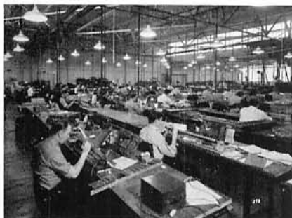
Relay mounting, spring adjusting and relay testing are done in this sub-assembly department. In the background are final finishing operations of switchboard plugs.
