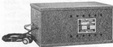
Type G full wave rectifier is designed for float charging small 16 to 24 volt batteries at rates up to .5 amperes. It consists of four small rectifier cells, transformer and
