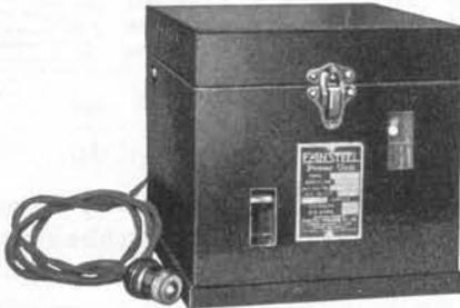
The CAB-4 power unit consists of a small Fansteel charger and a sealed type, 4-volt Exide battery, operating from 110-volt, 60-cycle A.C. current. It provides a constant battery supply for the operator's telephone circuit and night alarm, year after year without interruption. This is a popular unit with those who do not want to rely on dry cells or primary batteries.
