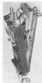
This type "H" protector unit is used in all apparatus of the Cook Trans-Mount system. Built on a strong, Bakelite base, it provides primary protection with a fuse and high-potential discharger and secondary high-potential protection after the fuse has blown.
