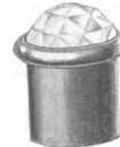
Type No. 9 lamp caps fits  $\frac{19}{32}$  inch holes. The nickel plated shank is  $\frac{7}{16}$  inch long. This cap is used generally for pilot and signal work.
