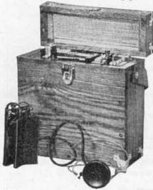
Locates high resistance water leaks, wet spots, shorts, crosses, and grounds. Locates the cable trouble to the inch. Equipped with exploring coil that will not pick up the tone on the sheath of cable due to its patented circuit that balances out the tone that carries past the trouble.
