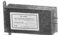
The No. 68 condenser is for use in older type magneto switchboard cord circuits. The can is  $3\frac{1}{8}$  inches long,  $1\frac{1}{2}$  inches wide and  $1\text{-}1/32$  inches thick. The working voltage is 400 volts direct current. Equipped with mounting ears.
