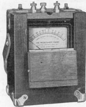
Direct reading resistance meter — enables the trouble man to make all tests for the detection, nature of the trouble and the approximate location of the fault either in the central office, on the line or at the subscriber's station.
