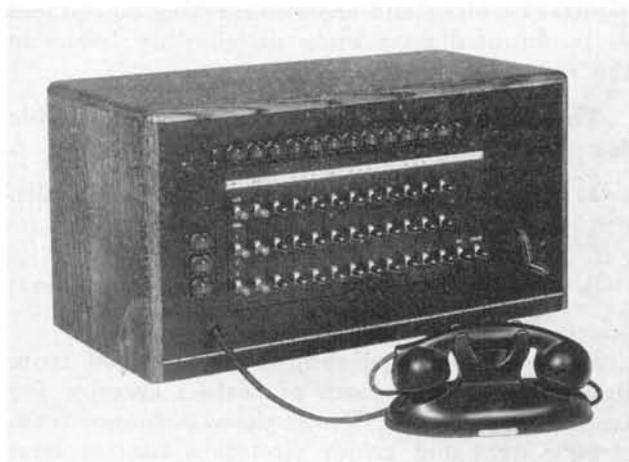
first key immediately under the line drop in the upward (listening) position. She is then connected with the calling party.
