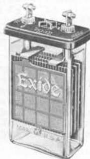
The elements are made up of plates of the pasted type, assembled with both wood and rubber separators in strong, sealed glass jars.
