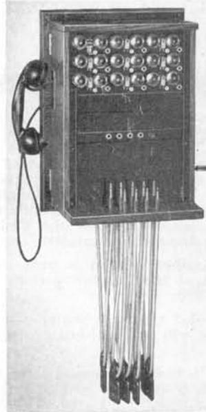
Here is an attractive wall switchboard designed especially for rural switching centers where the operator isn't always close to the board and a loud signal is desired. A double gong bell is wired across each line and operates similar to a telephone bell. These bells are located in the face of the switchboard, and through their code rings, the operator can tell at a distance whether a party line subscriber is signalling the operator or a subscriber on the same line.
