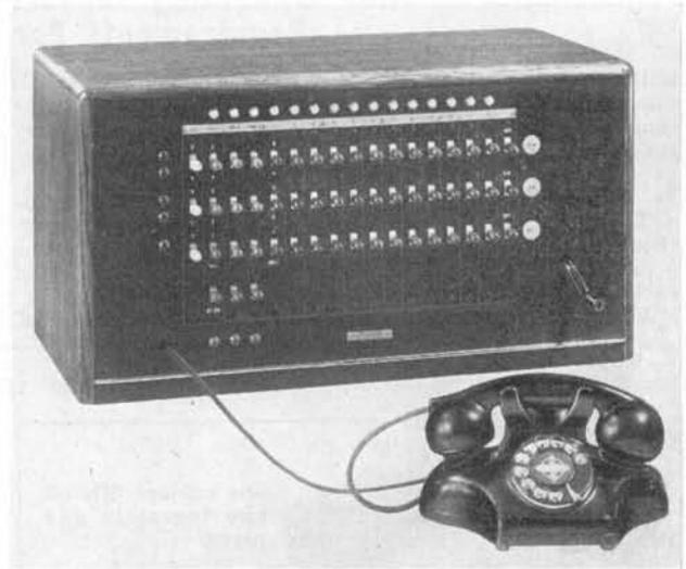
sers, fuse panel and connecting rack is mounted on a steel frame chassis which is fastened to the base board. The generator crank is in front.
