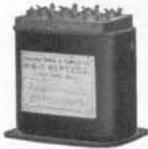
The No. 16-A repeating coil has the same electrical characteristics and uses as the No. 20-A but is designed to mount on wood. Made of two concentric wound coils, each coil being placed upon one leg of a horseshoe lamination. Resistance of windings are 20, 16, 20, 16 ohms respectively. Height  $3\frac{3}{4}$  inches, width  $3\text{-}21/32$  inches, length  $2\text{-}5/32$  inches. Net weight 3 pounds.
