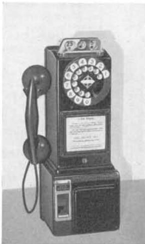
The dial of this station is normally inoperative until a coin is deposited. The deposited coin closes a switch which serves to unlock the dialing circuit so that a local call can be made. The deposited coin is held in suspension and through a special chain of relays in the central office, is automatically collected or refunded depending upon the completion or non-completion of the connection.
