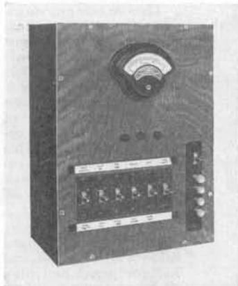
Every telephone exchange, large or small, magneto or common battery, should be equipped with good testing apparatus so that line, instrument or exchange troubles may be quickly and easily located. The Kellogg Junior Test Cabinet saves time and expense, and eliminates service interruptions. It is a small, compact unit suitable for mounting on or near the switchboard in small exchanges, or on the wire chief's desk in larger offices.
