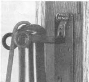
The principle of the Kellogg No. 1 battery saver is extremely simple. It stops the receiver hook after it has closed the receiver contact, but before the battery contact has been closed, thus permitting reception without the use of batteries. Pressing the stop lever releases the receiver hook which closes the battery contact permitting complete conversation. Net weight is 3 ozs.
