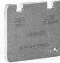
No. 50—Plug gauge for gauging worn No. 42 plugs.
