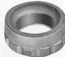
No. 71—For removing transmitter and receiver caps from F 27-C Masterphone handset.
