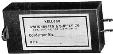
Code No. 28— \frac{1}{2} M. F. Dimensions No. 28, Height including terminals 2\frac{47}{64} in., Width, 1\frac{1}{4} in., Thickness, \frac{3}{4} in.
