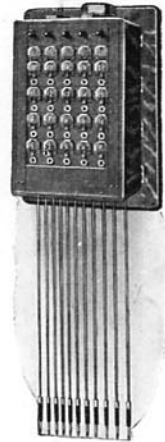
Kellogg 20 line wall switchboard with combined self-restoring drops and jacks, ringing and listening keys. Cabinet No. 11134.
