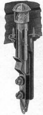
Fig. 150 Cross-section view of Lamp Jack mounting.
