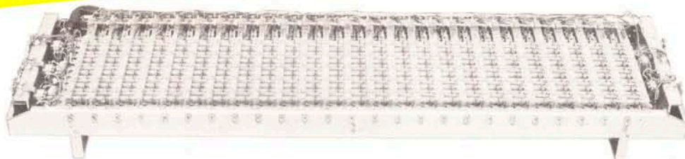
FIGURE No. 1 Kellogg Crossbar Switch
