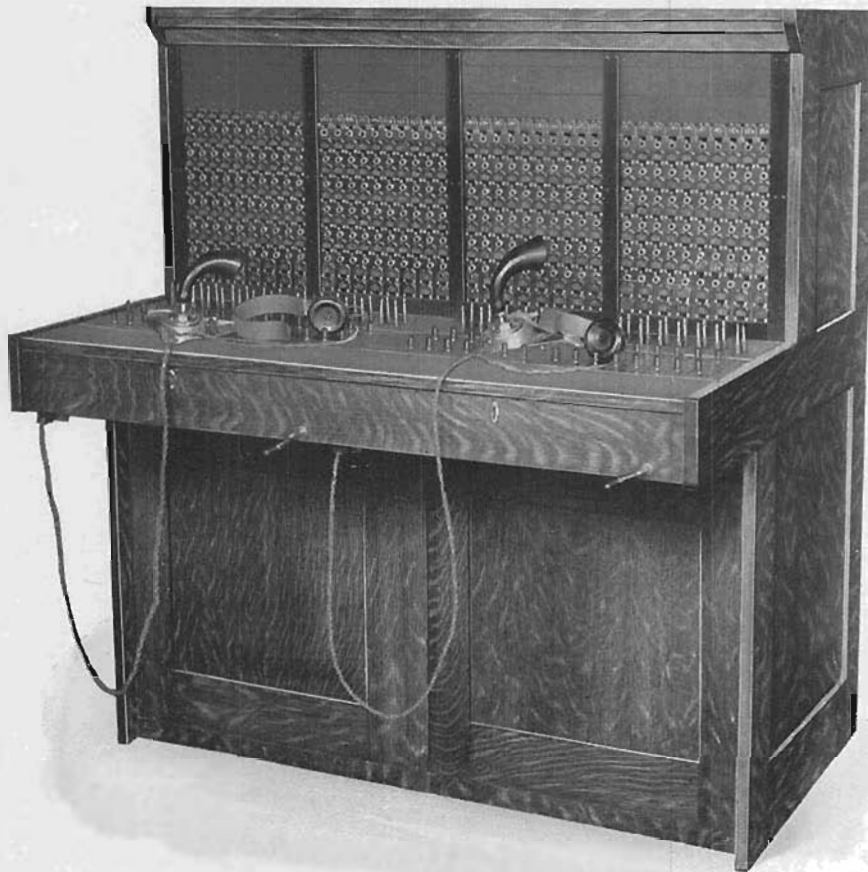
Fig. No. 108—Code No. 14-B—Wired for 240 lines, 30-cord circuits
