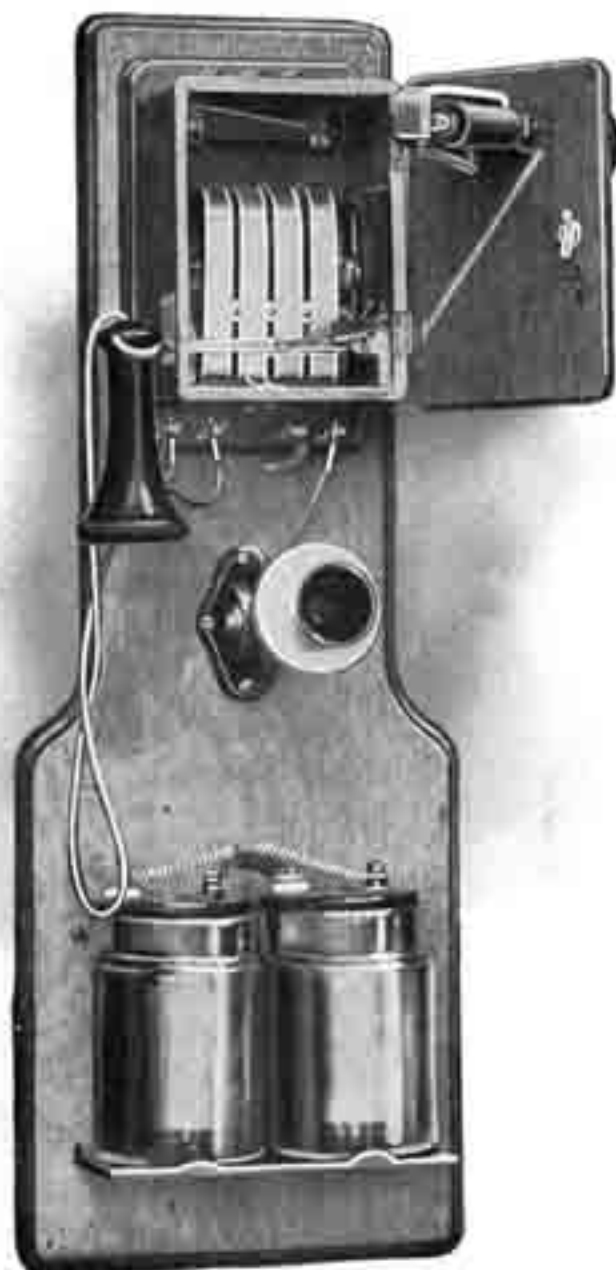
Bridging Telephone Opened
