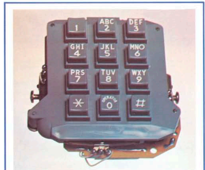
Type 35 —Identical to type 30 but has an additional set of normally open contacts for use with hands-free telephones. (Replaces type 28 dial.)
