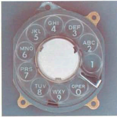
Type 10A —Miniature type with 2 3/8" numeral ring and automatic moveable finger stop. Designed for use in dial-in-handset telephones. Not provided with off-normal contacts.
