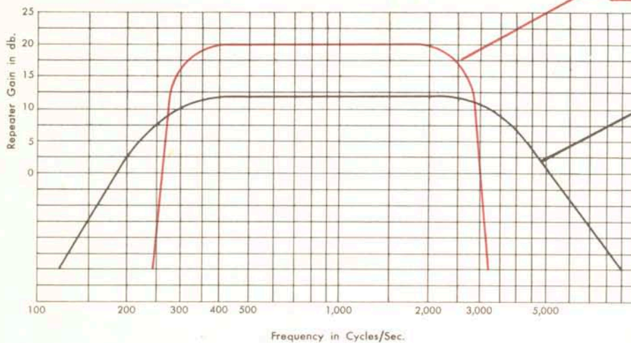
Frequency Response of Kellogg Telephone Repeaters #3A, #3B, and #4 Installed in an Average Toll Line
