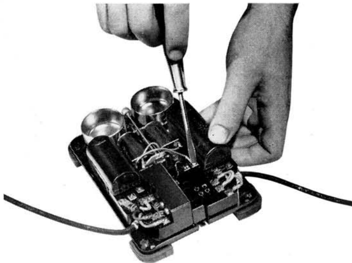
Figure 13 — Reversing Ringer Leads
