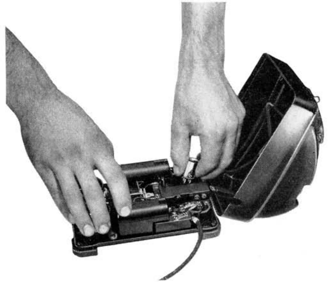
Figure 8 — Removing Dial Plug
