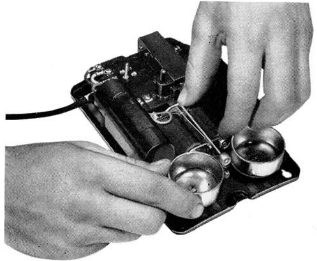
Figure 22 — Adjusting Gong Spacing
