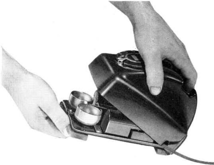
Figure 7 — Removing Desk Housing
