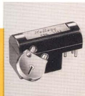
**Sealed-in Units**—The Condenser and Induction Coil are encased in individual moulded housings which are potted and sealed with moisture-proofing compound.
