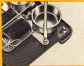
**Easy Accessibility**—two mounting screws are conveniently located and are easily removed with a medium-sized screw driver.
