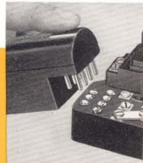
**Plug-in connection**—The Condenser and Induction Coil plug into pin jacks on the Interconnecting Block in the same manner as you plug in a radio tube.
