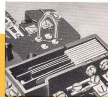
**Switch Assembly**—All moving parts of the switching mechanism, including the spring stack-up, are housed in a dust-proof compartment on the interconnecting block. The twin-contact, nickel-silver spring leaves, are directly connected with the permanent wiring of the Universal circuit.
