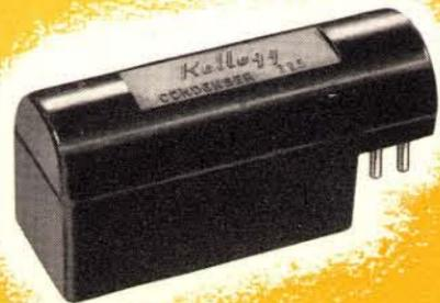
**UNIVERSAL CONDENSER** A single condenser unit is used for all circuit applications. This condenser provides the necessary capacity for the talking circuits and by means of a switching unit on the inter-connecting block, provides either 0.5 or 1.0 MFds. of capacity as required by the ringer used.
