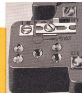
**Condenser Control Switch**—a slide-link on the interconnecting block provides either 0.5 MF or 1.0 MF of capacity as required in the ringing circuit.
