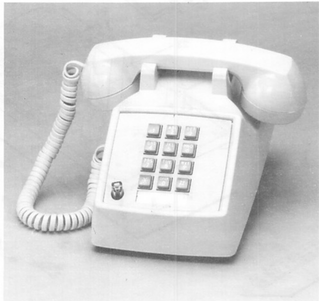
Figure 1: 2-Line, Pushbutton Dial, Desk Telephone
