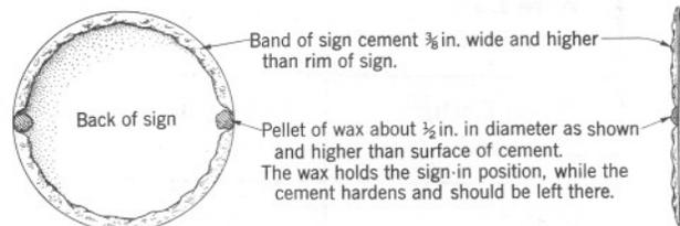
10. Cemented signs may be removed by carefully chipping out the cement between the sign and mounting surface. Chip around the entire circumference until sign is loosened. Do not pry sign off as this may damage mounting surface.
