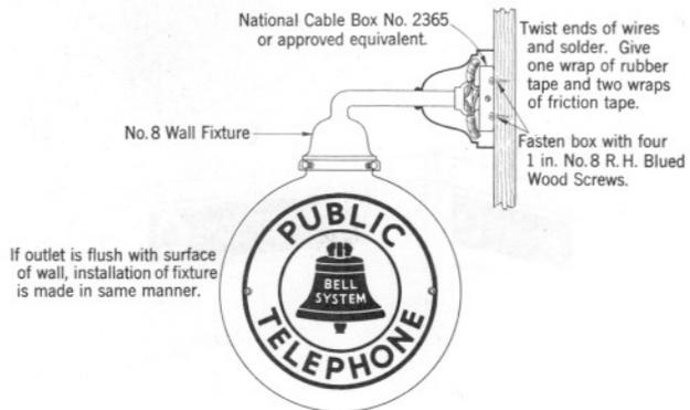
Fig. 13 – No. 8 Sign – Wall Installation
