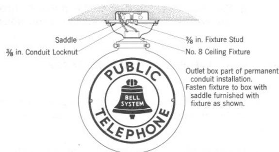
Fig. 15 — No. 8 Sign — Ceiling Installation — Other Surfaces
