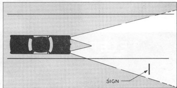
**Fig. 18 – Correct and Incorrect Locations for the KS-16540 Sign**
