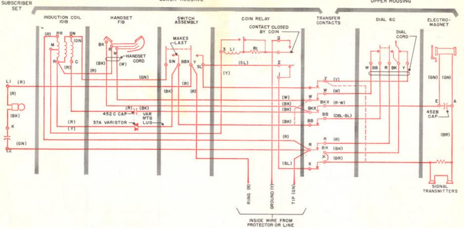
Note 1: Dotted lines in diagram show manual set connections.
