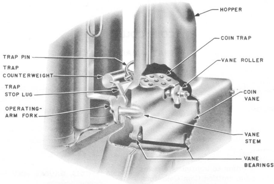
Fig. 2 — Hopper and Rear of Coin Relay
