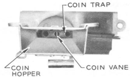
**Fig. 10 — Position of Vane When Relay is Centered**
